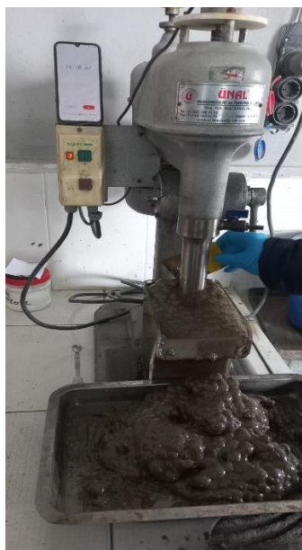
Figure 2. Foam formation during the flotation process
